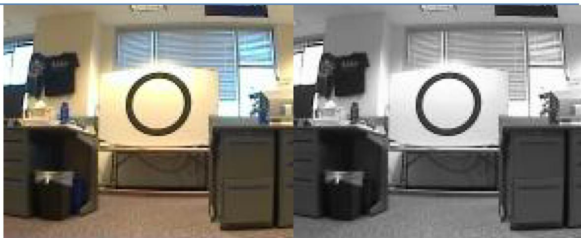
Above are two images, the first a color image taken with the camera on the robot as recorded by the driver station. The second image was produced by extracting the luminance plane from the first image leaving only greyscale.
