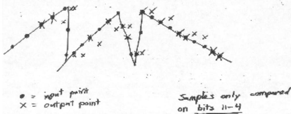
Figure 17: 3 Point Average Reject Filter
